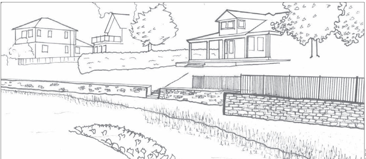
Waves and boat wakes can erode sediment from underneath a seawall and undermine the wall's structural integrity over time. Natural breakwaters such as oyster reefs and restored shoreline vegetation can help protect against this "scour."
