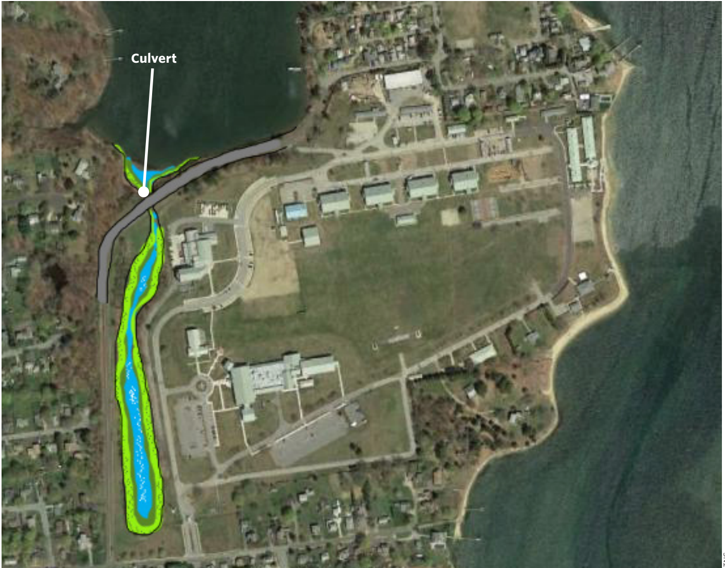
Installing a culvert beneath Pine Grove Road can connect tidal flow to an existing wetland on Army National Guard land. This would help to clean water entering the cove and increase salt marsh habitat in the River over time.
