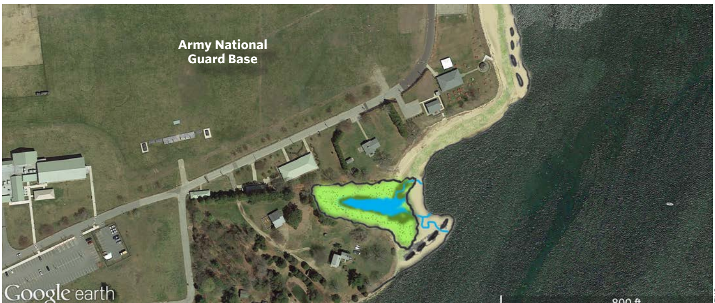
An oyster reef and re-vegetated edge with native plant species can further enhance shoreline stabilization efforts at the Army National Guard Base. There may also be space along this shoreline to accommodate salt marsh advancement.
