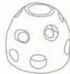
Reef balls can attenuate 30% of wave energy (Mattei, 2017).
