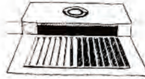
Catchment basin/ storm drain
